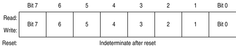
Figure 10-15. TIM Channel 1 Register Low (TCH1L)
