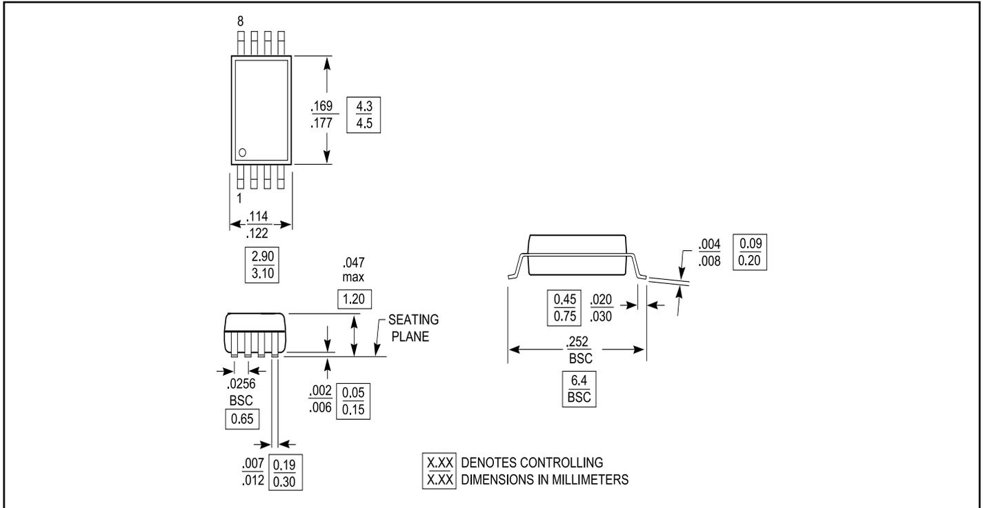
**Packaging Mechanical: 8-Pin MSOP (U)**
