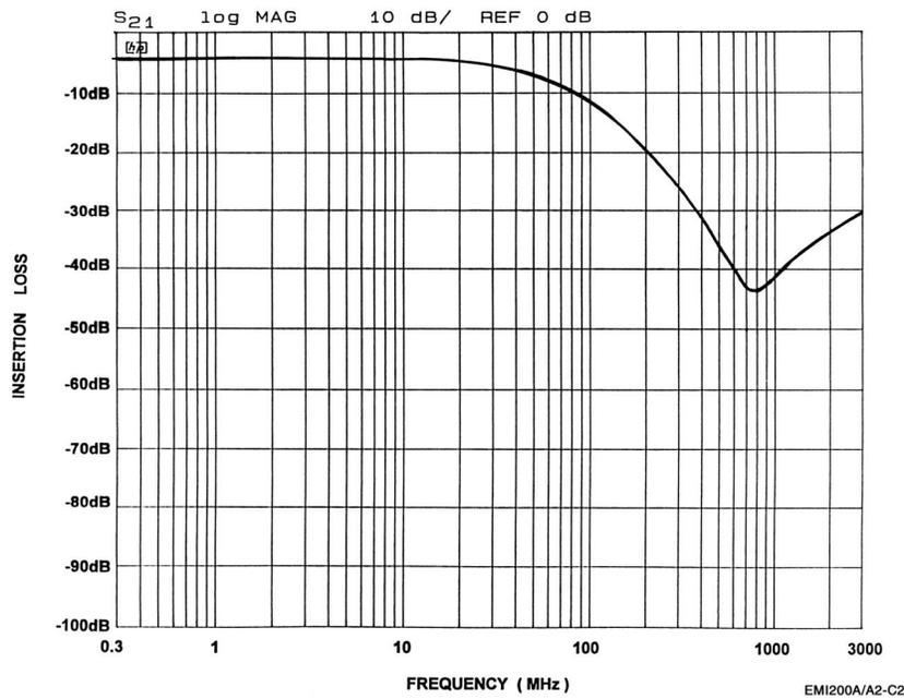
**Figure 2. Microphone 2 Circuit (A2-C2) EMI Filter Performance**
