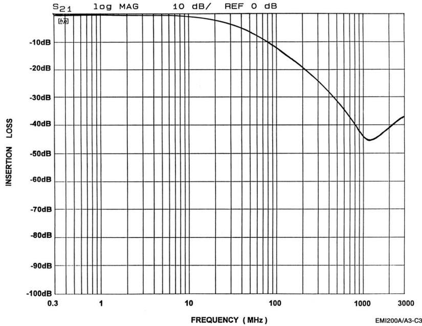
**Figure 3. Speaker 1 Circuit (A3-C3) EMI Filter Performance**
