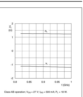
Fig.10 Load impedance as a function of frequency (series components); typical values.
