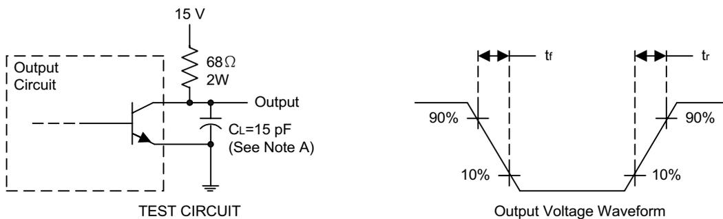
NOTE A. CL includes probe and jig capacitance.
