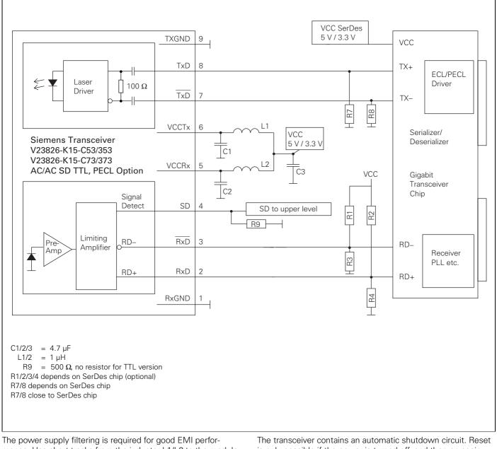
mance. Use short tracks from the inductor L1/L2 to the module  $V_{CC} Rx/V_{CC} Tx.$
