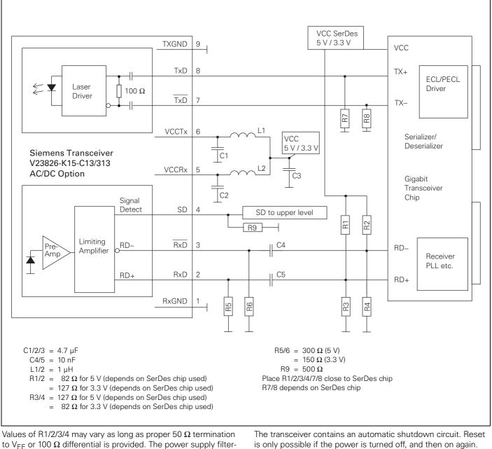
ing is required for good EMI performance. Use short tracks from the inductor L1/L2 to the module V<sub>CC</sub>Rx/V<sub>CC</sub>Tx.
