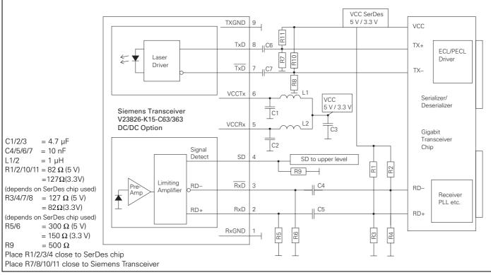
Values of R1/2/3/4 may vary as long as proper 50  $\Omega$  termination to V<sub>EE</sub> or 100  $\Omega$  differential is provided. The power supply filtering is required for good EMI performance. Use short tracks from the inductor L1/L2 to the module V<sub>CC</sub>RX/V<sub>CC</sub>TX.
