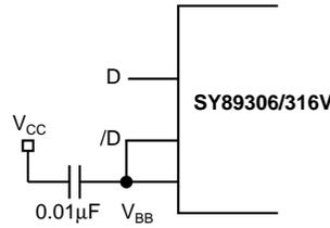
**Figure 1. Single-Ended LVPECL Input (Terminating Unused Input)**
