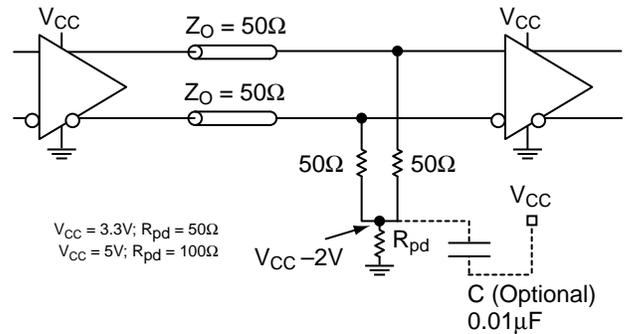
**Figure 2b. Three Resistor "Y Termination"**
