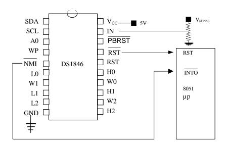
$$V_{SENSE} = \frac{R1 + R2}{R2} \ X \ 1.25 \qquad \qquad V_{MAX} = \frac{V_{SENSE}}{V_{TP}} \ X \ V_{CC}$$
