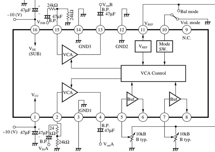
1. Voltage of Pin 7 becomes center at  $1/2 V_{REF}$  in case of using at balance mode.
