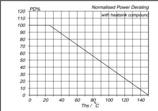
Fig.11. Normalised power dissipation.  $PD\% = 100 \cdot P_D/P_{D.25^{\circ}C}$
