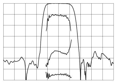
Horizontal: 3 MHz/div Vertical (from top): Magnitude 10,1 dB/div Phase Deviation 10 deg/div Group Delay Variation 200 ns/div
