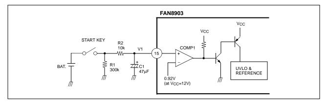
In the state of the start-key turned off, all the blocks in the FAN8903 are kept to be off because the power is not supplied into UVLO&REFERENCE block.
