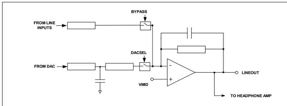
**Figure 8 Line Output Schematic**
