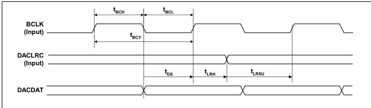
Figure 3 Digital Audio Data Timing – Slave Mode
