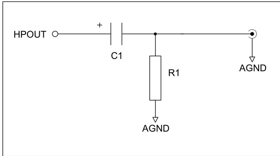
**Figure 11 Headphone Output Application Drawing**
