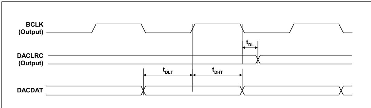
Figure 2 Digital Audio Data Timing - Master Mode
