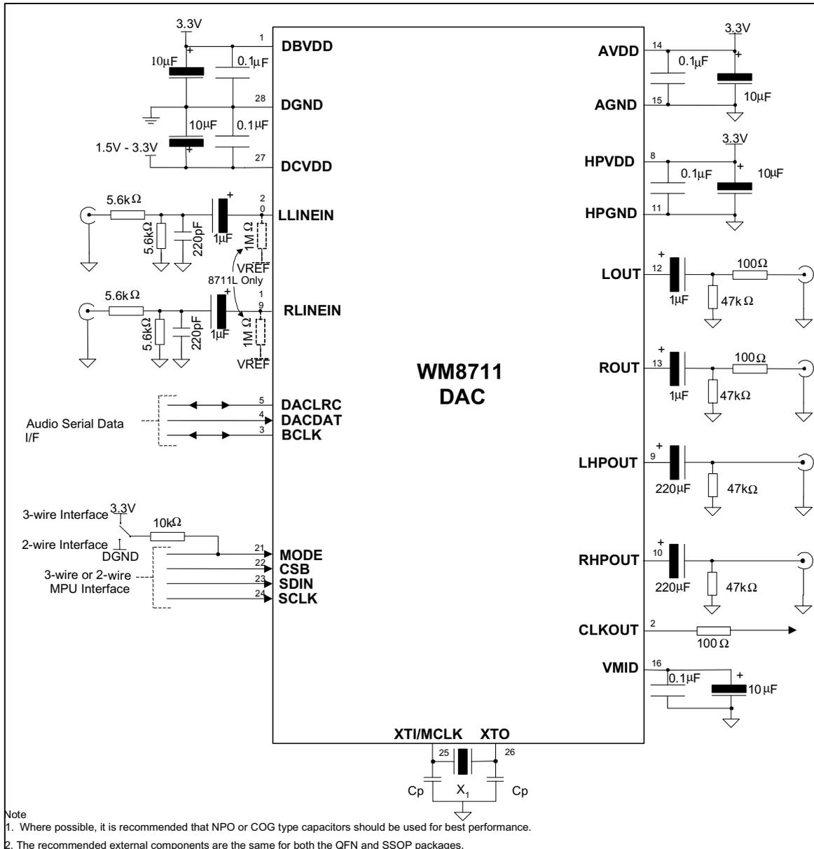
Figure 35 External Components Diagram
