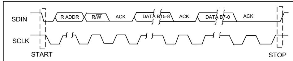
**Figure 20 2-Wire Serial Interface**
