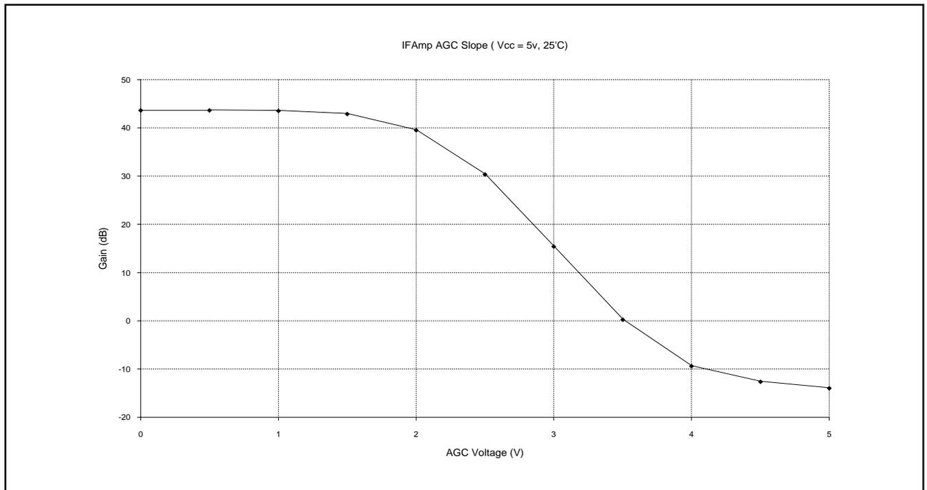
Figure 7 - Typical IF amplifier stage AGC characteristic
