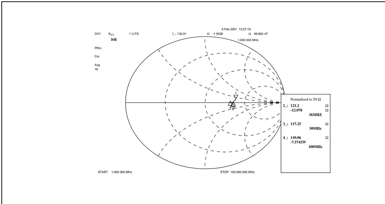
Figure 6 - Typical SAWF driver output impedance, single-ended
