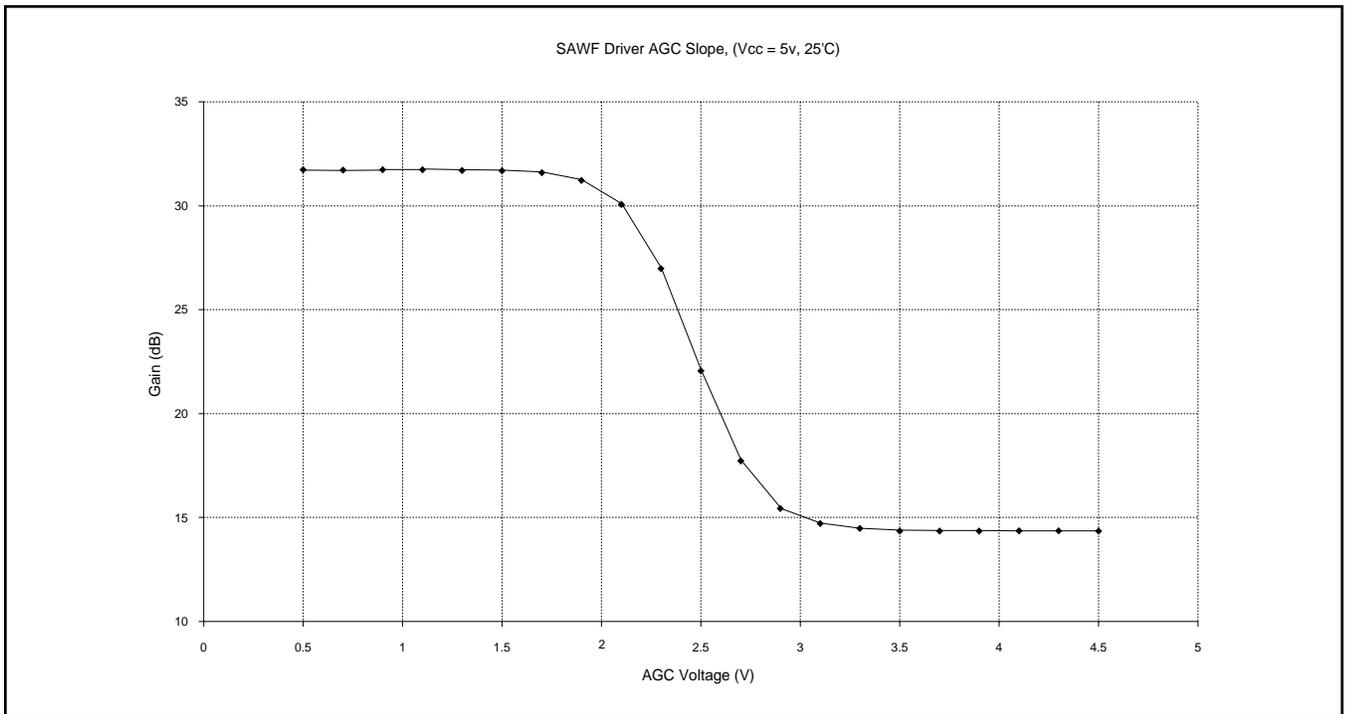
Figure 3 - Typical SAWF driver stage AGC characteristic
