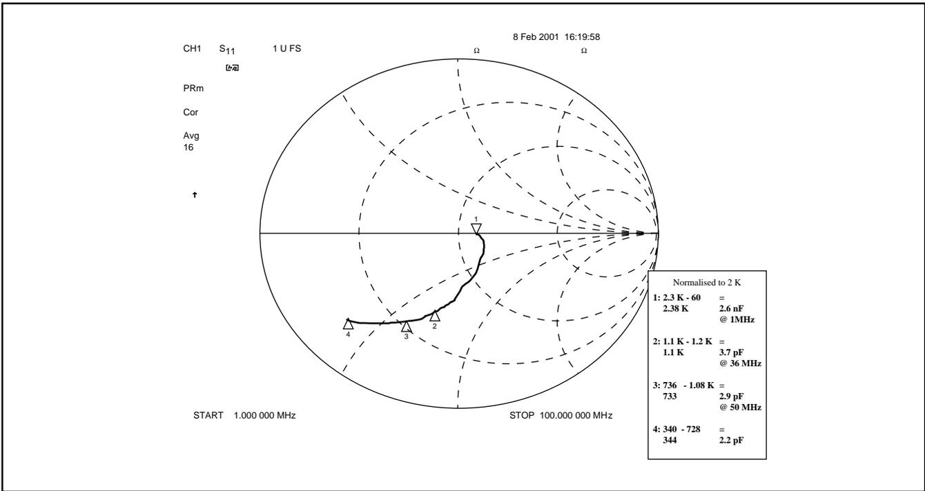
Figure 8 - Typical IF amplifier input impedance, single-ended
