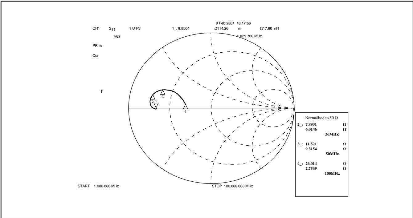
Figure 9 - Typical IF amplifier output impedance, single-ended
