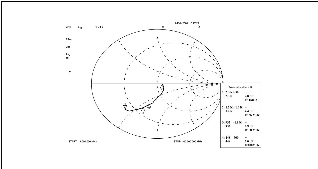
Figure 5 - Typical SAWF driver input impedance, single-ended
