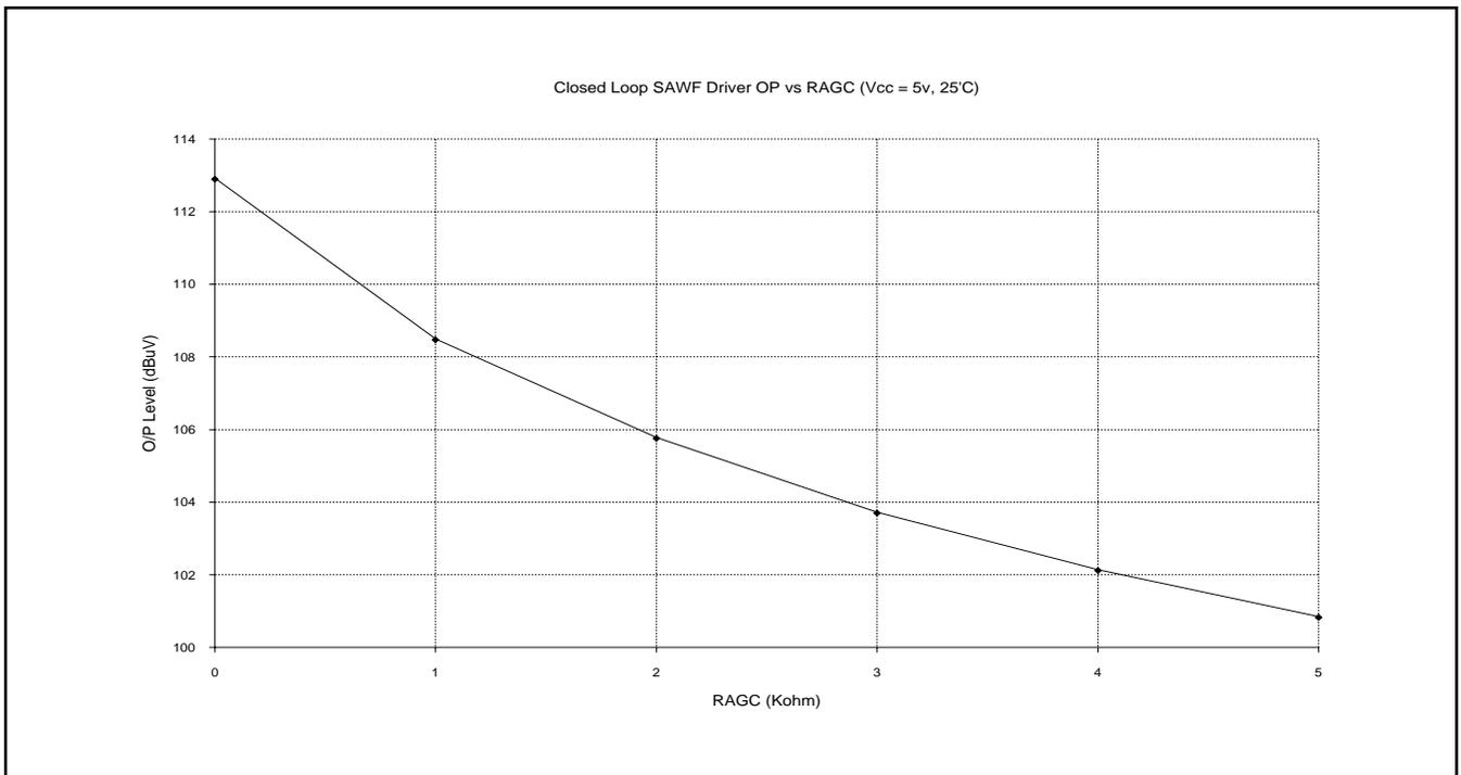
Figure 4 - AGCOUT characteristic versus AGCBIAS resistor
