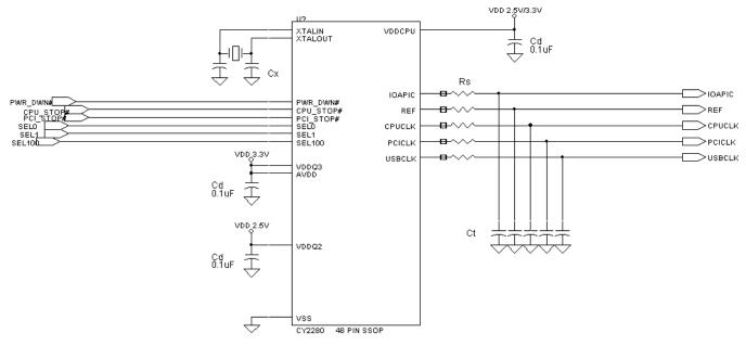
Crt. = DECOUPLING CAPACITORS
