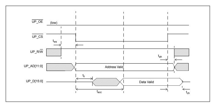
Figure 23 - CPU Interface Motorola Timing - Read Access
