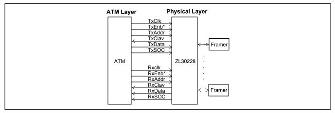
Figure 12 - ATM Interface to ZL30228
