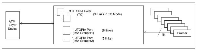
Figure 14 - ATM Mixed-Mode Interface to One ZL30228
