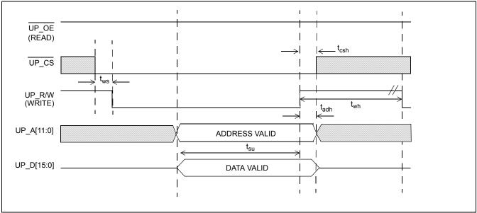
Figure 26 - CPU Interface Intel Timing - Write Access
