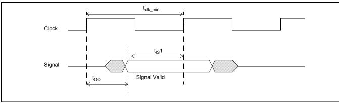
Figure 20 - Output Delay Timing
