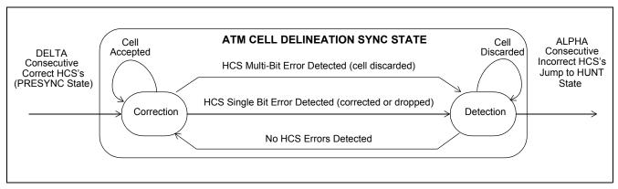
Figure 8 - SYNC State Block Diagram
