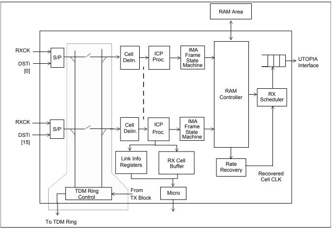
Figure 9 - ZL30228 Receiver Circuit in IMA Mode
