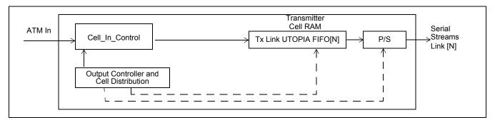
Figure 6 - Functional Block Diagram of the Transmitter in TC Mode
