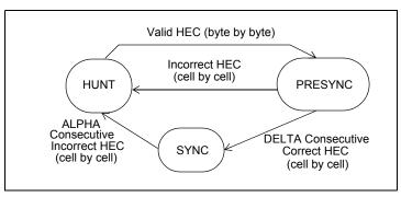
Figure 7 - Cell Delineation State Diagram
