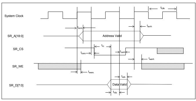
Figure 21 - External Memory Interface Timing - Read Cycle
