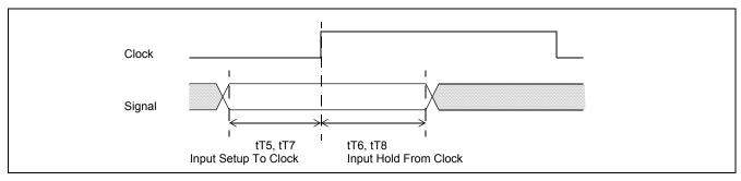
Figure 18 - Setup and Hold Time Definition
