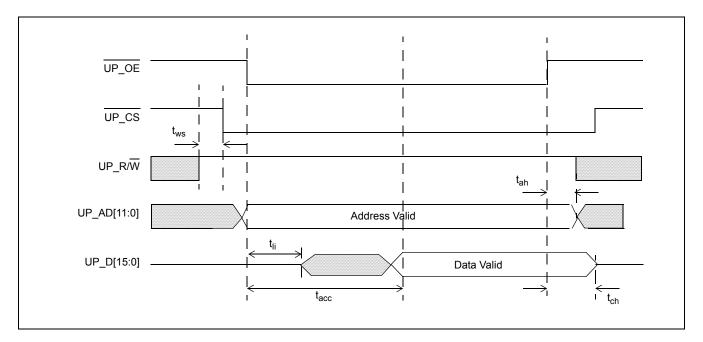
Figure 24 - CPU Interface Intel Timing - Read Access
