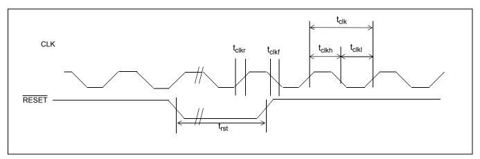
Figure 31 - System Clock and Reset
