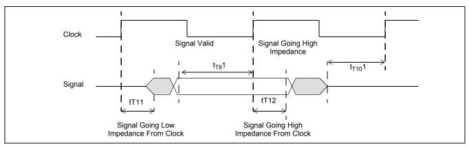
Figure 19 - Tri-State Timing
