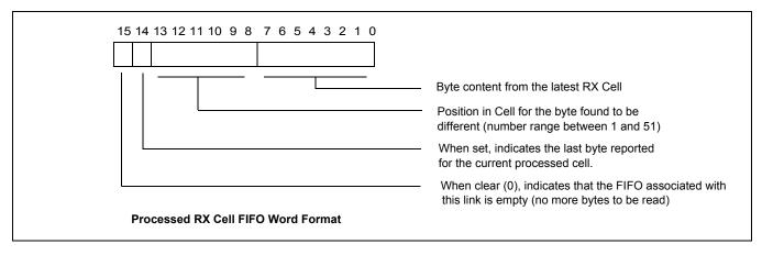
Figure 16 - Processed RX Cell FIFO Word Format
