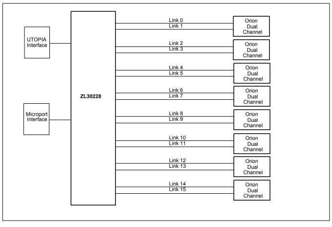
Figure 17 - Interface to SHDSL Device
