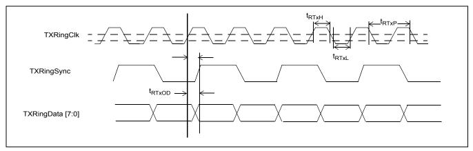
Figure 28 - TDM Ring TX Timing Diagram
