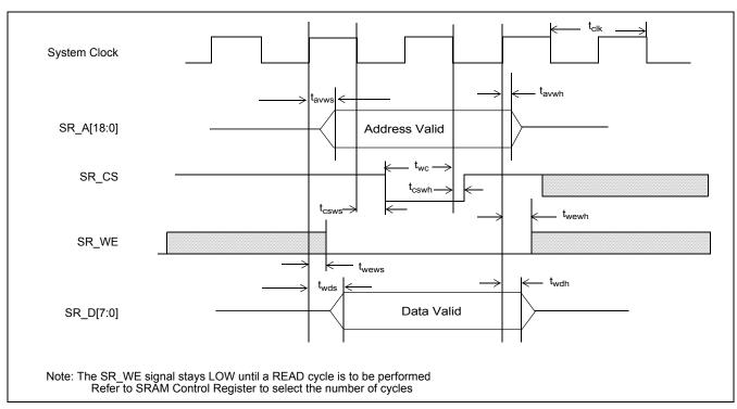
Figure 22 - External Memory Interface Timing - Write Cycle
