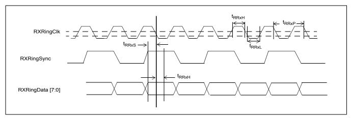
Figure 29 - TDM Ring RX Timing Diagram
