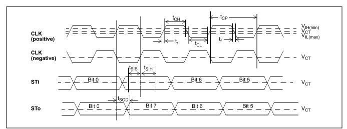
Figure 27 - Serial TDM Bus Timing
