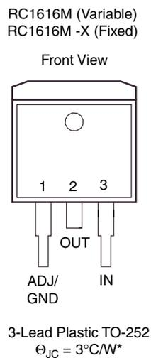
\*With package soldered to 0.5 square inch copper area over backside ground plane or internal power plane,  $\Theta_{JA}$  can vary from  $30^{\circ}\text{C/W}$  to  $>50^{\circ}\text{C/W}$ . Other mounting techniques may provide better power dissipation than  $30^{\circ}\text{C/W}$ .
