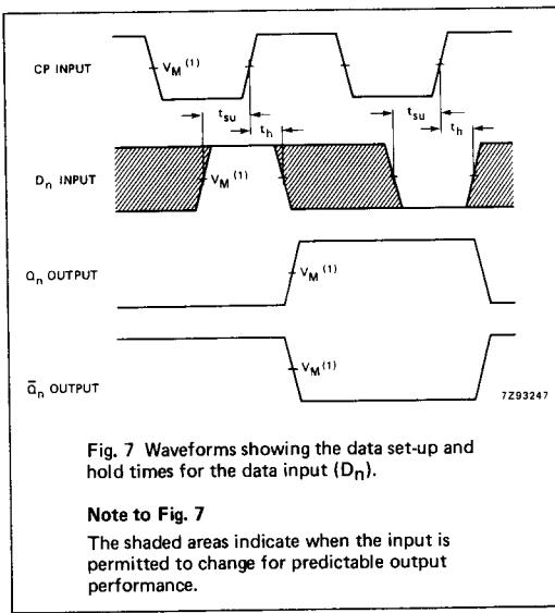
Fig. 7 Waveforms showing the data set-up and hold times for the data input ( $D_n$ ).
