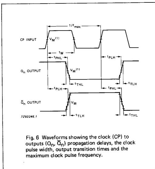
Fig. 6 Waveforms showing the clock (CP) to outputs ( $Q_n$ ,  $\bar{Q}_n$ ) propagation delays, the clock pulse width, output transition times and the maximum clock pulse frequency.
