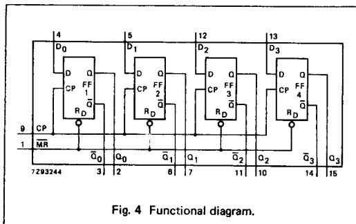
Fig. 4 Functional diagram.
