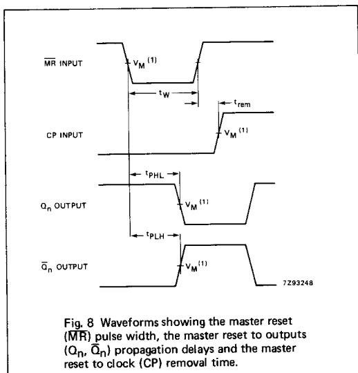
Fig. 8 Waveforms showing the master reset (MR) pulse width, the master reset to outputs ( $Q_n$ ,  $\bar{Q}_n$ ) propagation delays and the master reset to clock (CP) removal time.
