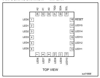
Figure 2. Pin configuration — HVQFN
