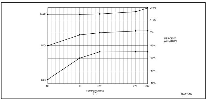
Figure 16. Typical frequency variation over process at  $V_{DD}$  = 2.3 V to 3.0 V
