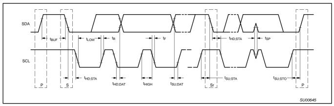
Figure 19. Definition of timing
