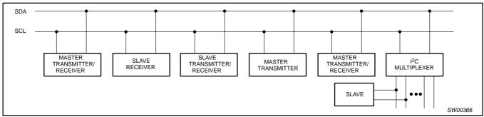
Figure 8. System configuration
