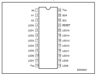
Figure 1. Pin configuration — SO, TSSOP
