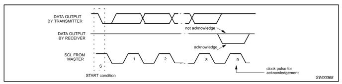
Figure 9. Acknowledgement on the I<sup>2</sup>C-bus
