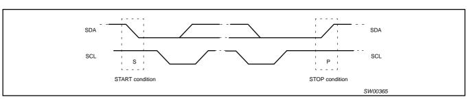
Figure 7. Definition of start and stop conditions
