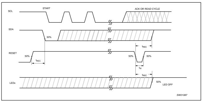
Figure 18. Definition of RESET timing
