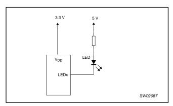
Figure 15. Device supplied by a lower voltage
