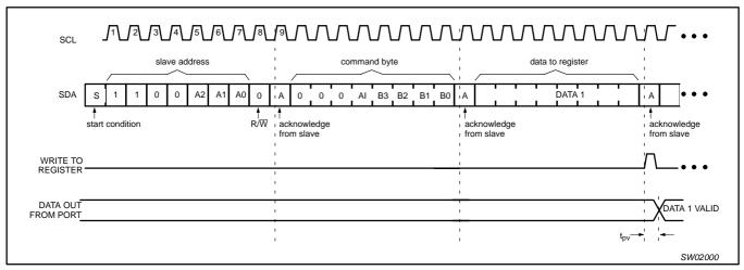
Figure 10. WRITE to register
