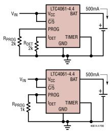
Figure 6. Two Circuits That Charge at 500mA Full-Scale Current and Terminate at 50mA
