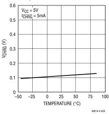
ACPR Pin Output Low Voltage vs Temperature
