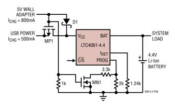
Figure 8. Combining Wall Adapter and USB Power
