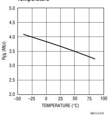
C/5 Pin Pulldown Resistance vs Temperature
