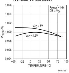
PROG Pin Voltage vs V<sub>CC</sub> (Constant-Current Mode)
