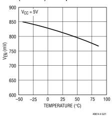
C/5 Pin Threshold Voltage (High-to-Low) vs Temperature
