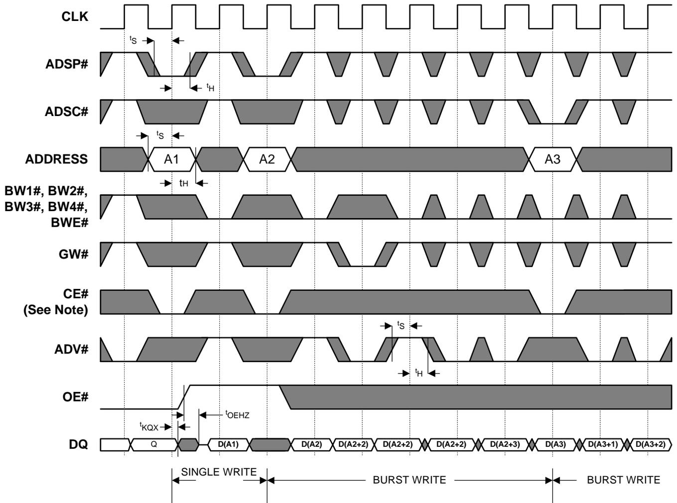
Note: CE# active in this timing diagram means that all chip enables CE#, CE2, and CE2# are active.
