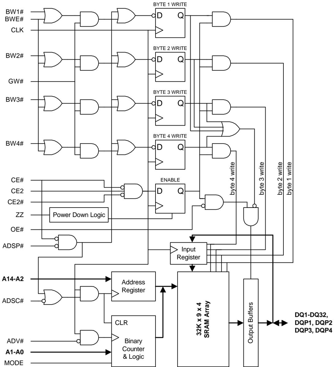
**NOTE:** The Functional Block Diagram illustrates simplified device operation. See Truth Table, pin descriptions and timing diagrams for detailed information.
