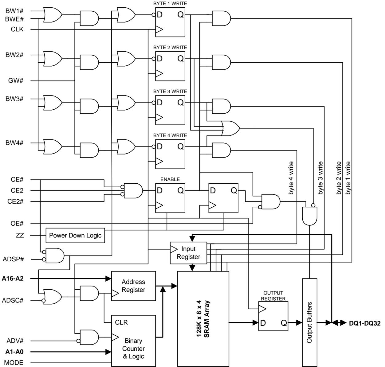
**NOTE:** The Functional Block Diagram illustrates simplified device operation. See Truth Table, pin descriptions and timing diagrams for detailed information.
