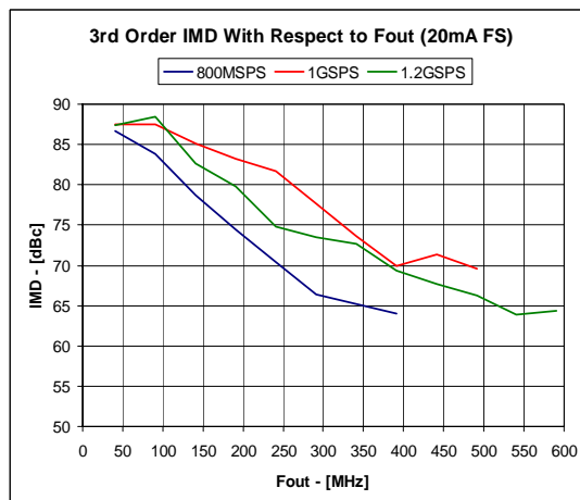
TPC3. AD9736, 3 rd Order IMD vs. Fout and Sample Rate
