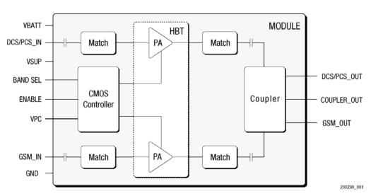
Figure 1. SKY77331 Functional Block Diagram
