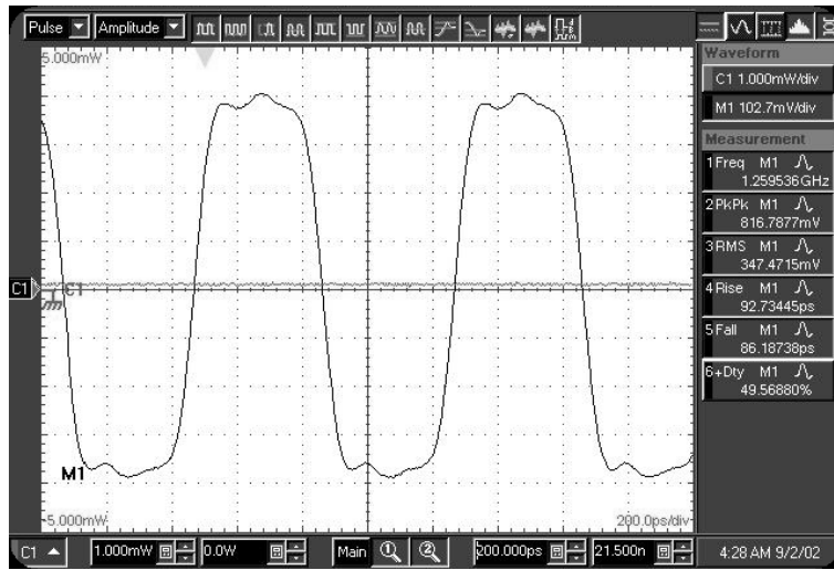
Figure 12 - Differential output with small input amplitude waveform V_{CC} = 4.75V , V_{in} = 10dBm , F_{in} = 5GHz
