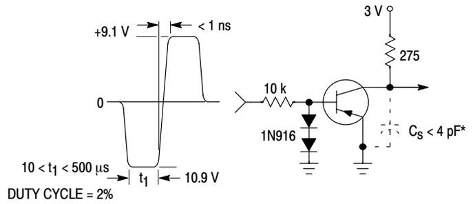
**Figure 2. Storage and Fall Time Equivalent Test Circuit**
