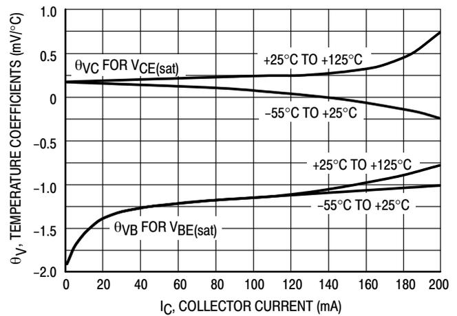
Figure 16. Temperature Coefficients
