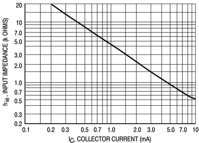
Figure 11. Input Impedance
