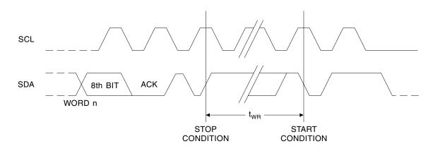
Note: The write cycle Time  $t_{WR}$  is the time from valid stop condition of a write sequence to the end of the internal clear/write cycle.
