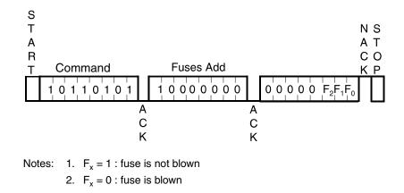
The Read Fuses operation is always allowed. The device only transmits one data byte and waits for a new command.
