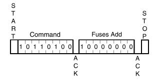
The Write Fuses operation is only allowed under secure code control and no data byte is transmitted by the host. The fuses are blown sequentially: CMA is blown if FAB is equal to "0", and PER is blown if CMA is equal to "0". If the fuses are all 0's, the operation is canceled and the device waits for a new command.
