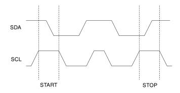
Note: The SCL input should be LOW when the device is idle. Therefore, SCL is LOW before a start condition and after a stop condition.
