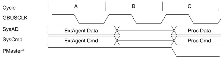
Figure 6.3.5 Sample Cycle with **PMaster\*** Asserted
