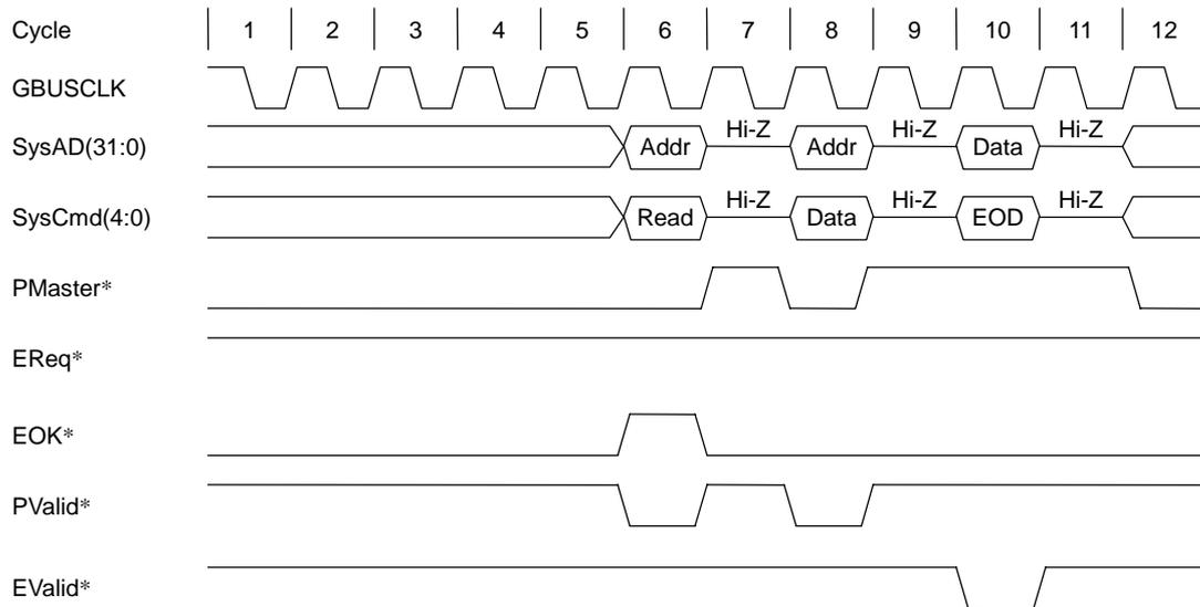
Figure 6.3.31 Discarding and Re-executing Processor Single Read Request
