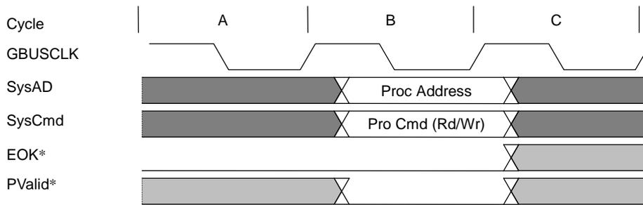
Figure 6.3.8 Sample Cycle with **EOK\*** Asserted
