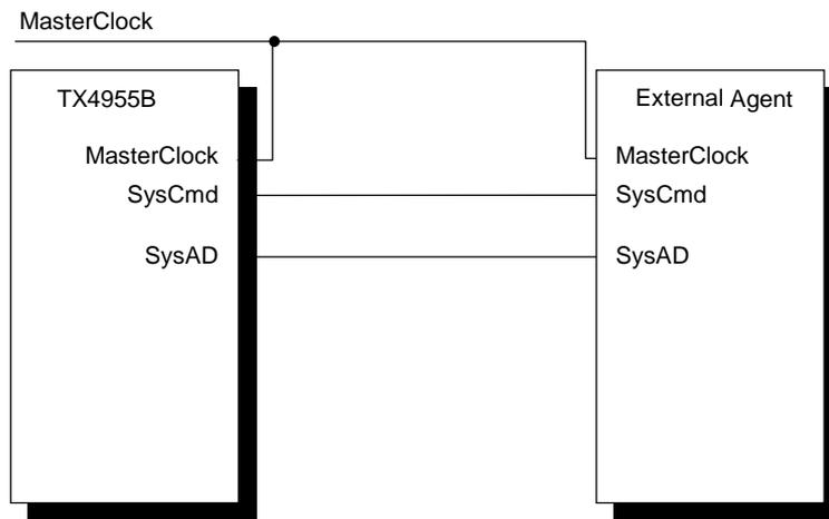
Figure 4.3.1 The TX4955B Processor Phase-Locked System
