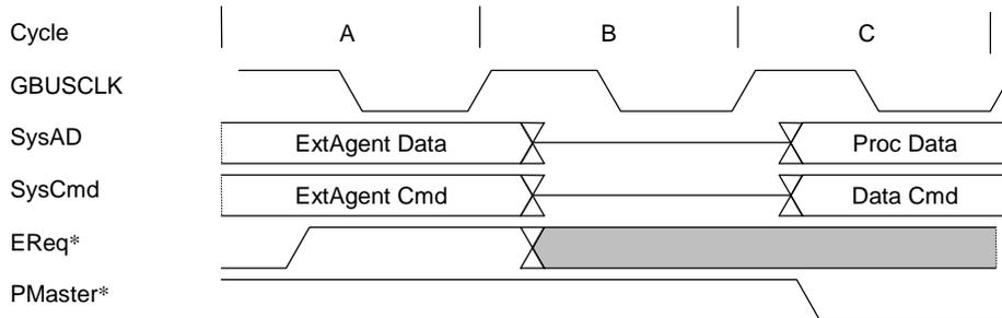
Figure 6.3.11 Sample Cycle with Deassertion of **EReq\***
