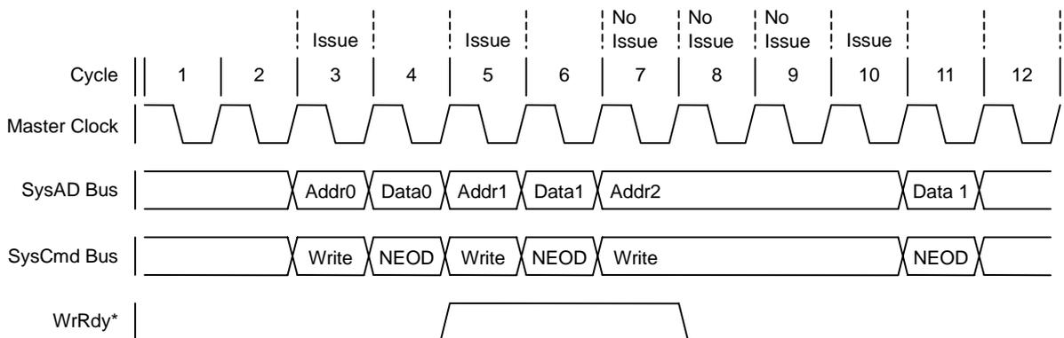
Figure 6.2.16 Pipeline Write Protocol
