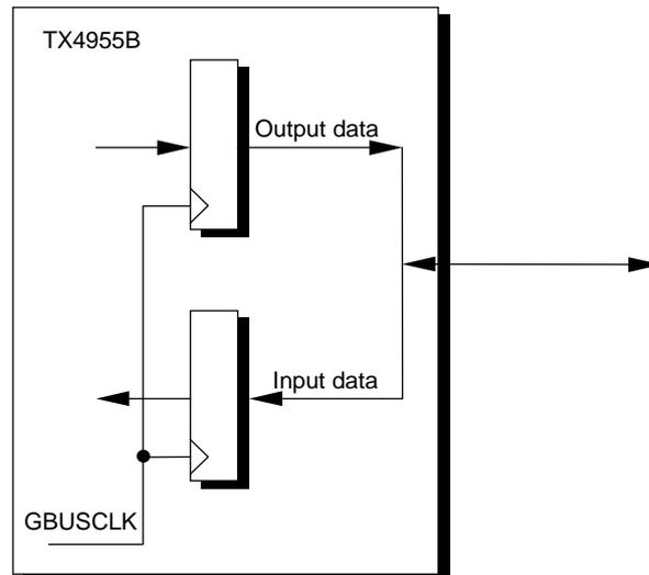
Figure 6.3.2 System Interface Register-to-Register Operation
