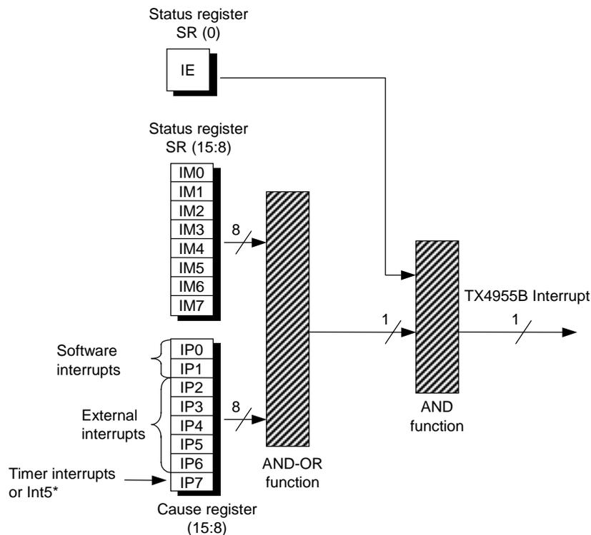
Figure 8.5.1 Masking of the TX4955B Interrupts
