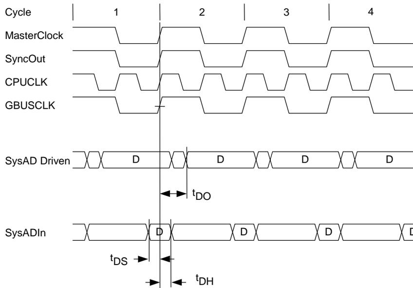
Figure 4.2.2 Processor Clock, CPUCLK-to-GBUSCLK Divisor of 2
