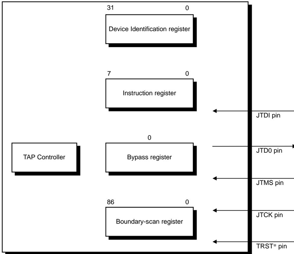
Figure 7.2.1 JTAG Interface Signals and Registers
