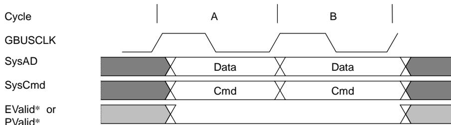
Figure 6.3.7 Sample Cycles with Multiple **PValid\*** and **EValid\***
