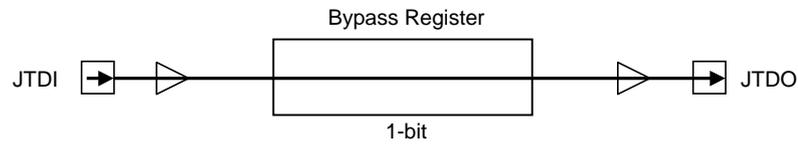
Figure 7.4.4 Test Data Flow While the Bypass Instruction is Selected
