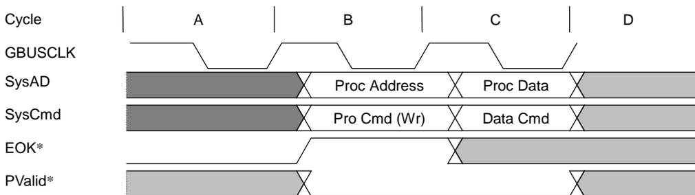
Figure 6.3.9 Sample Cycle with **EOK\*** Asserted, Then Deasserted
