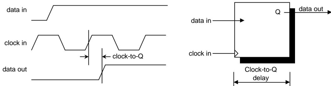
Figure 4.1.2 Clock-to-Q Delay
