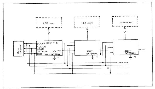
\*1: In this example, "H" is output by the positive logic, that is, when "H" is written from DATA IN, "H" is output with a LOAD signal. If the OSC pin is connected to VDD, the output has the negative logic, that is, the logic level input from the DATA IN pin is inverted and output.
