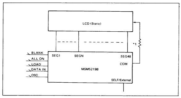
\*1: When this IC is used under a strong external noise or large-capacity LCD load, this resistor prevents latch-up to be caused by a low output impedance of the COM pin. The resistance is about  $100\Omega$ .
