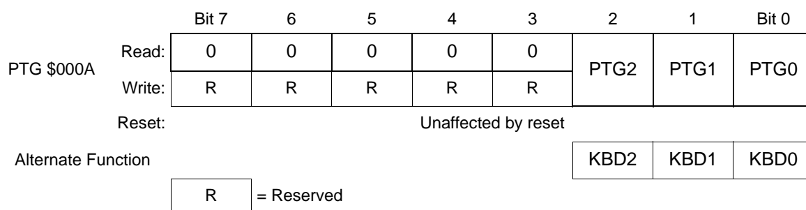
Figure 19-19. Port G Data Register (PTG)
