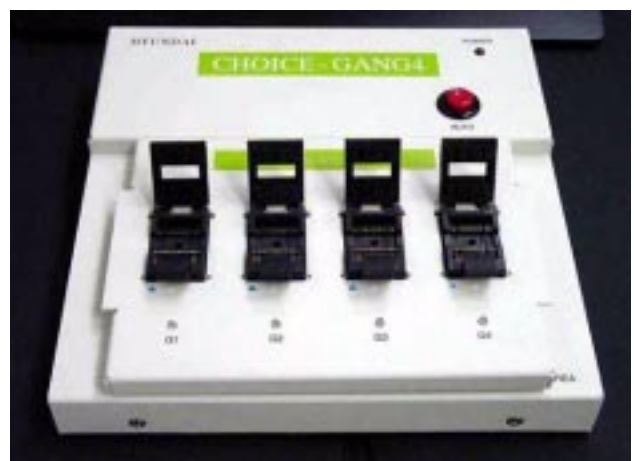
Figure 1-3 OTP Gang Programmer CHOICE-GANG4™
