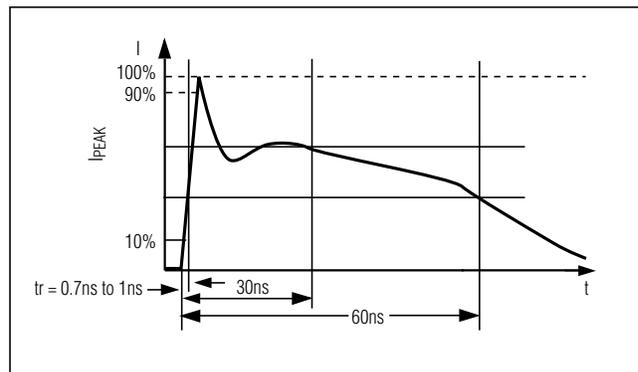
Figure 6b. IEC 1000-4-2 ESD Generator Current Waveform
