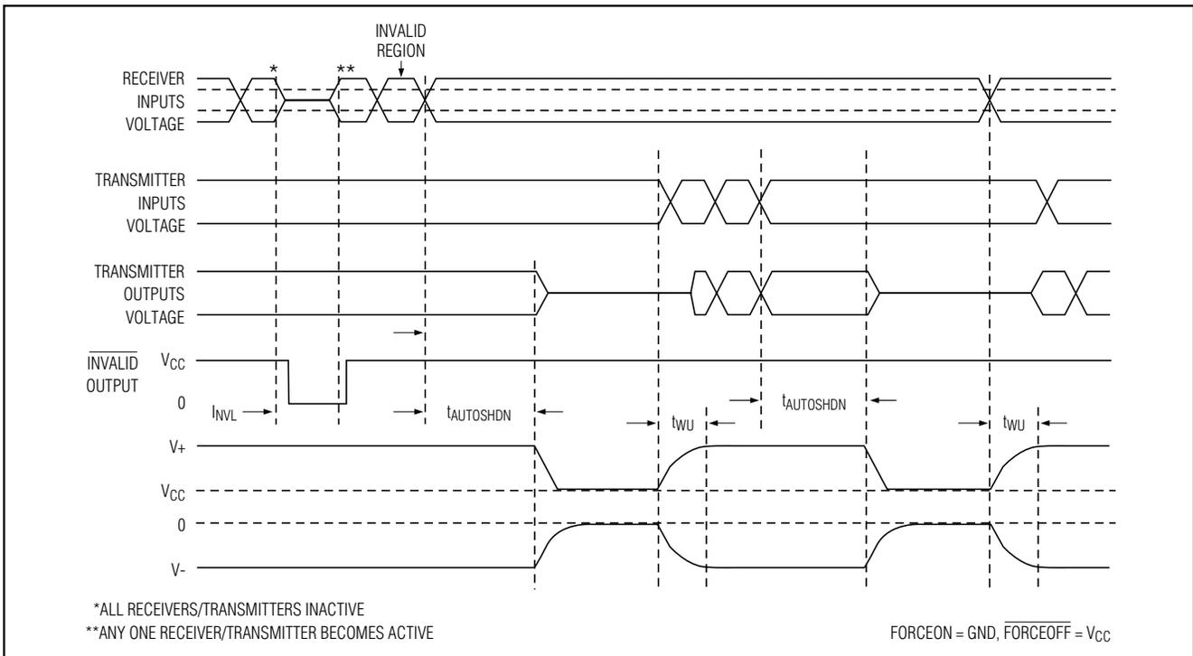
Figure 4b. AutoShutdown Plus and  $\overline{\text{INVALID}}$  Timing Diagram
