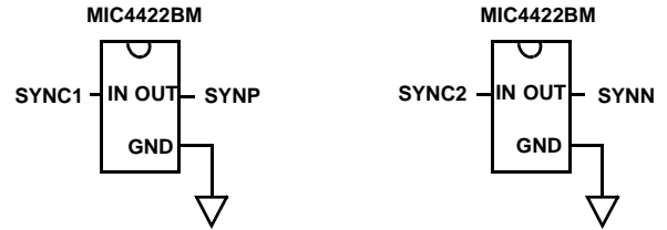
FIGURE 22B. NON-INVERTING DRIVERS
