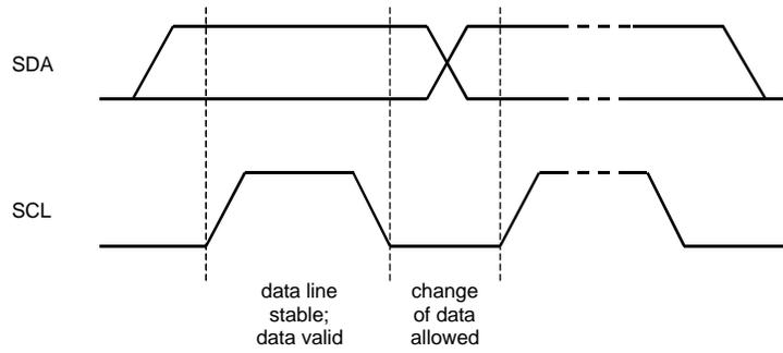
Figure 16. Bit transfer on the I<sup>2</sup>C-bus
