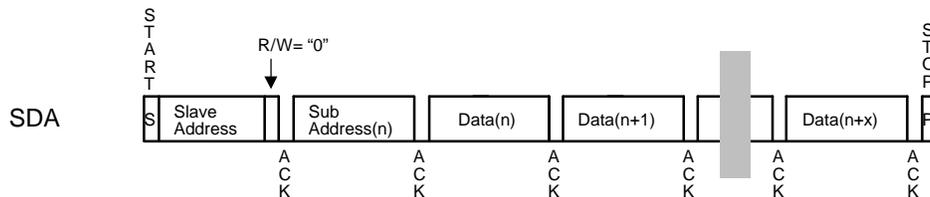
Figure 8. Data transfer sequence at the I<sup>2</sup>C-bus mode
