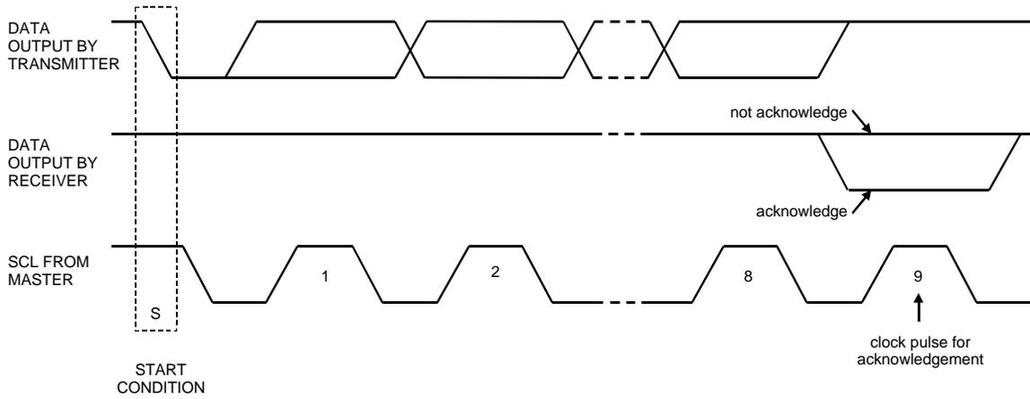
Figure 15. Acknowledge on the I<sup>2</sup>C-bus
