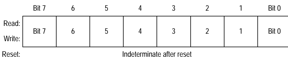
Figure 10-13. TIM Channel 0 Register Low (TCH0L)
