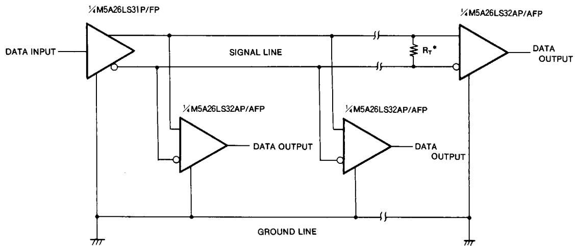
$R_T^*$  = Characteristic impedance of transmission line.
