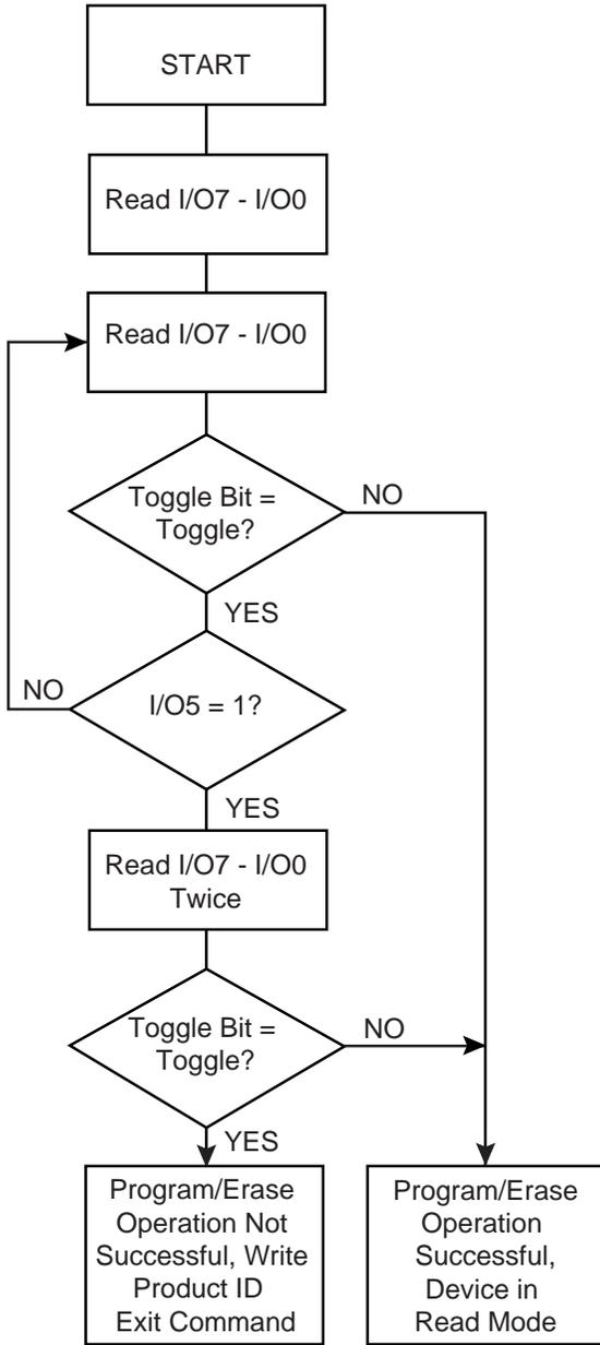
**Figure 4.** Toggle Bit Algorithm
