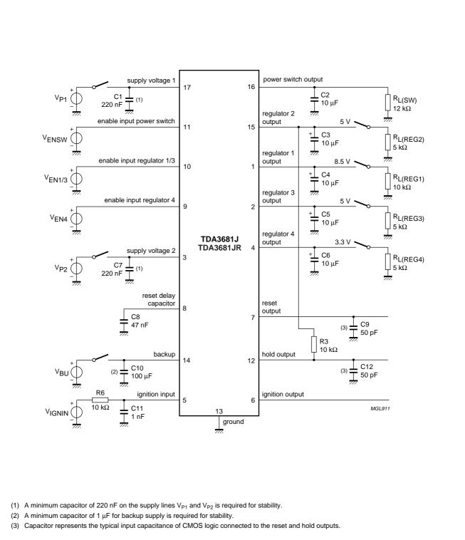
Fig.10 Test circuit of TDA3681J and TDA3681JR.
