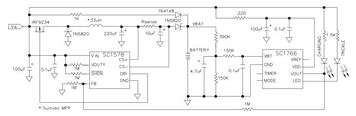
NOTE: RSENSE = 0.1 ohm, CHARGE CURRENT = 0.5A  $\pm 10\%$ ,  $V_{IN} > V_{BAT} + 3.5V$  RSENSE = 0.05 ohm, CHARGE CURRENT = 1.0A  $\pm 10\%$ ,  $V_{IN} > V_{BAT} + 4.0V$  RSENSE = 0.033 ohm, CHARGE CURRENT = 1.5A  $\pm 10\%$ ,  $V_{IN} > V_{BAT} + 4.5V$  EFFICIENCY > 90%, MEASURED AT CS- NODE
