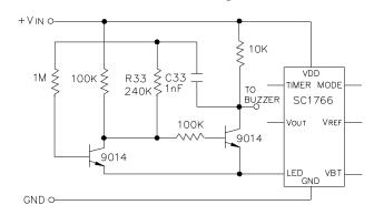
NOTE: Frequency (about 1Hz) is determined by R33 and C33. Buzzer will be activated when LED pin goes low.
