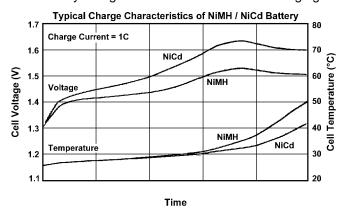
takes only 1 hour or less with a simple control circuit. One main purpose of the control circuit is to terminate the fast charge process to prevent the temperature and internal pressure of the battery cell from building to a damaging level which degrades or even destroys the battery cell.
