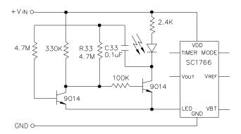
NOTE: Frequency (about 1Hz) is determined by R33 and C33. LED will flash when LED pin goes low.
