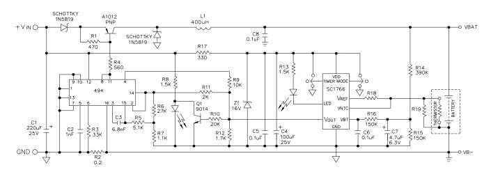
NOTE:  $+V_{IN}$  should be higher than 10V. Z1 is required when  $+V_{IN}$  exceeds 18V. Fast charge current is approximately 1A, adjustable through R7. Trickle charge current is adjustable through R12.
