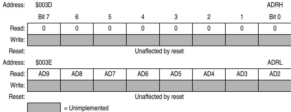
Figure 5-7. ADC Data Register High (ADRH) and Low (ADRL)
