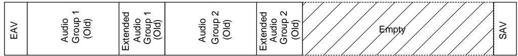
Video signal after GS9023 Removal of Audio Group 1 & Extended Audio Group 1 (ANCI = LOW or "VSEL" = HIGH and "ADEL" = LOW)
