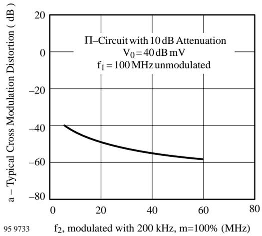
Figure 3. Typ. Cross Modulation Distortion vs. Frequency  $f_2$
