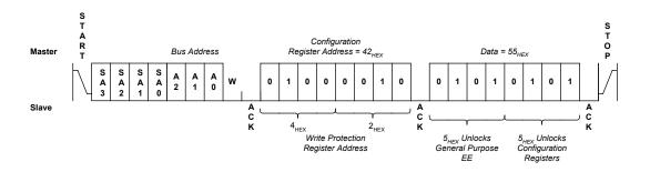
Figure 9 - Write Protection Register Write
