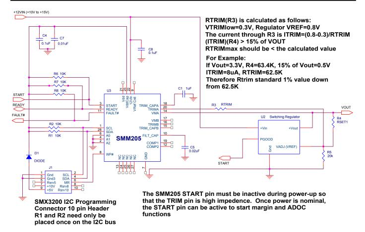
Figure 7 – SMM205 Applications schematic for an adjustable switching regulator (Full regulator circuit not shown).
