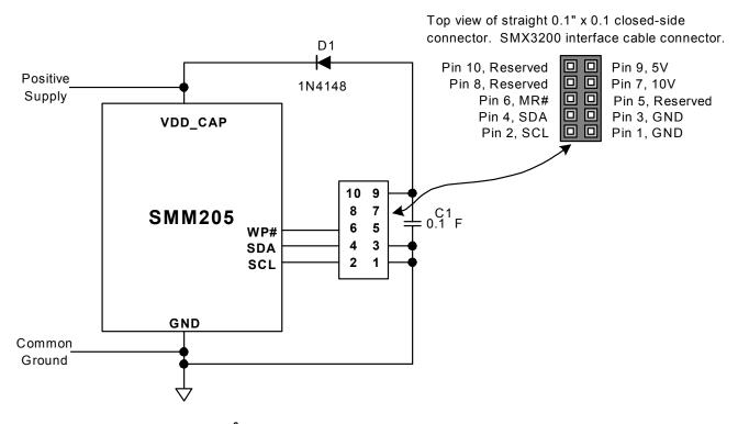
Figure 8– SMX3200 Programmer  $I^2C$  serial bus connections to program the SMM205. The SMM205 has a Write Protect pin (WP#) which, when asserted, prevents writing to the configuration registers and EE memory. In addition, there is a configuration register lock bit which, once programmed, does not allow the configuration registers to be changed.
