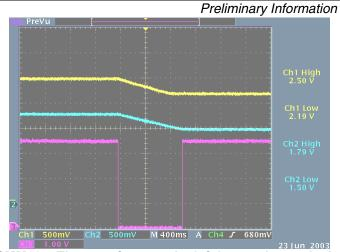
Figure 2 – Example Power Supply Margining using the SMM205. The waveform on the left is margin nominal to high from 2.5V to 2.8V and 1.8V to 2.1V. The waveform on the right is margin nominal to low from 2.5V to 2.2V and 1.8V to 1.5V. The bottom waveform is the READY signal indicating when margining is complete.
