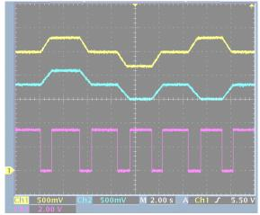
Figure 5 – SMM205 margin example. The nominal setting for channel 1 and 2 is 2.5V and 1.8V. The device margins the DC/DC converters from nominal to high (2.8V and 2.1) then to nominal, then to low (2.3V and 1.5V), then to nominal, then to channel 1 high and channel 2 low, and then back to nominal. The READY signals goes low when margining and high when complete.
