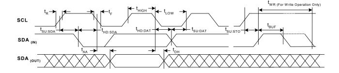
Figure 4 . Basic I<sup>2</sup>C Serial Interface Timing
