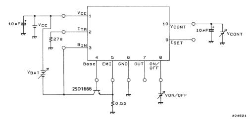
**Equivalent Circuit Block Diagram and Peripheral Circuit Example** (Values are reference values)
