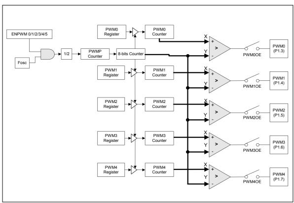
FIGURE 1 PWM DIAGRAM
