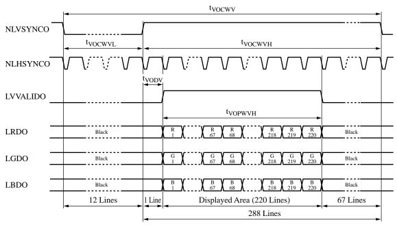
Note) When V\_POS = 1, line 0 and lines 221 to 287 will be filled with black in the LCD RGB, and only lines 1 to 220 will be output.
