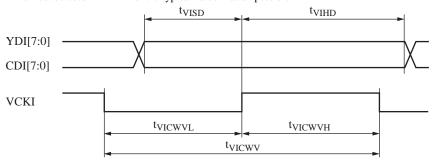
Figure 1. YC data input timing
