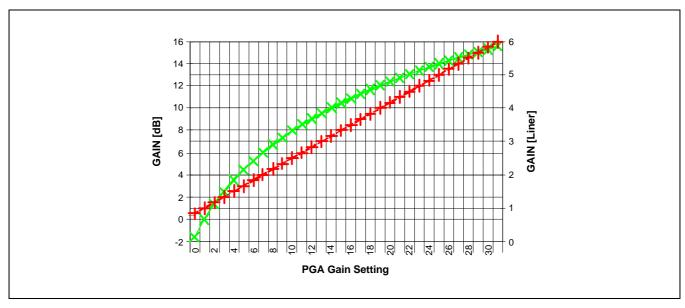
There is a gain boosting block before 12-bit ADC, which can muliply PGA's output signal by 1.5 (3.5dB) or pass it. This is controlled by gain mode of configuration register.
