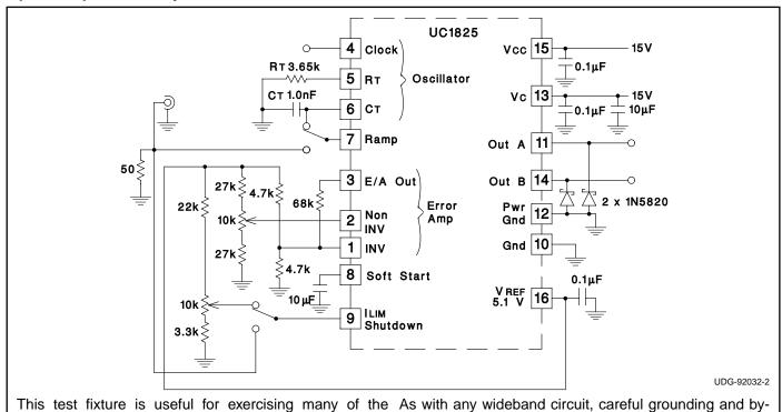
UC1825's functions and measuring their specifications. pass procedures should be followed. The use of a ground plane is highly recommended.
