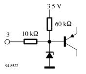
Figure 6. Input selector switch (Pin 3)
