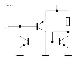
Figure 11. Tuner AGC – output (Pin 11)
