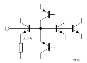
Figure 15. Internal reference voltage (Pin 17)
