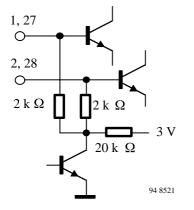
Figure 5. Sound IF inputs (Pin 1-2, 27-28)
