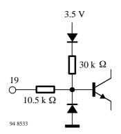
Figure 17. AFC switch (Pin 19)
