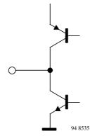
Figure 19. AFC output (Pin 22)
