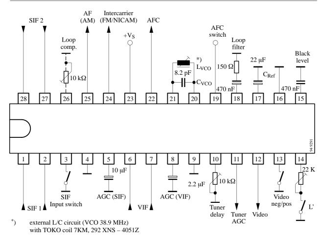
Figure 3. Test circuit
