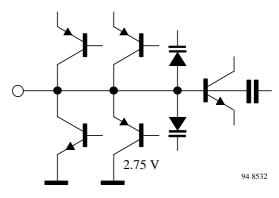
Figure 16. Loop filter (Pin 18)
