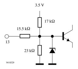
Figure 13. Standard switch (Pin 13)
