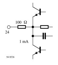
Figure 20. Intercarrier output (Pin 24)
