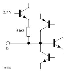
Figure 14. Black level capacitor (Pin 15)
