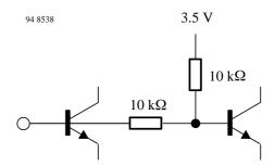
Figure 22. VCO offset compensation (Pin 26)
