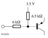
Figure 10. Tuner AGC - take over point (Pin 10)
