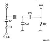
C1 and R1: Used for oscillator stabilization.
